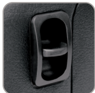
COMPRESSOR SWITCH/AIR RELEASE VALVE
