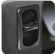
COMPRESSOR SWITCH/AIR RELEASE VALVE
