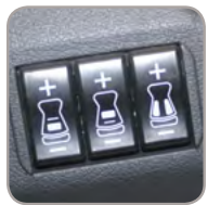
ADJUSTABLE AIR LUMBAR & AIR BOLSTERS
