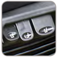
ADJUSTABLE HEIGHT, DAMPER, & SEAT TILT
