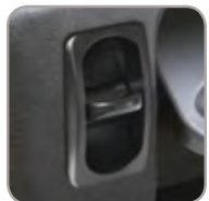
COMPRESSOR SWITCH/AIR RELEASE VALVE
