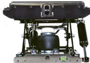
Double Damper View
