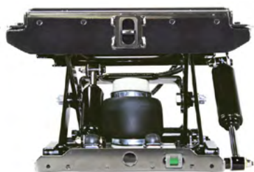
Double Damper View
