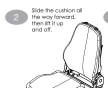
Slide the seat pan forward and back to access the mounting holesto install the OEM CAT bracket.
